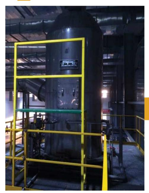
As parts of our equipment, we also provide washer exhaust acid mist neutralizing tower and decorator/base coat mist collector. The Neutralizing tower equipped with monitor, automatic add chemicals and water, achieve AUTO.
